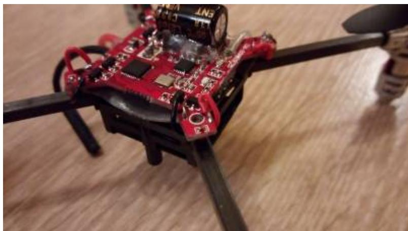
I had to cut down the edges to fit under the Canopy. That causes losing the LEDs.
