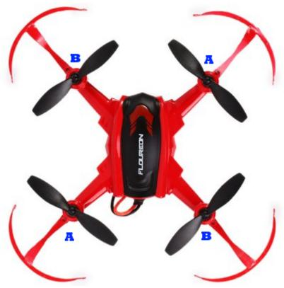
2. Motors/properliers are obstructed in some way. Check each propeller is spinning freely when flicked with your finger. Any that do not spin freely are at issue. Check that these are not pressed too firmly causing friction between the frame and the propeller. Also check for foreign objects such as hair or cobwebs, etc.
