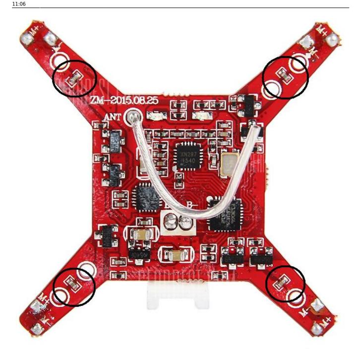
Don't forget to set the output signal polarity in the firmware, each method requires a different output signal polarity, because the signal is inverted when it passes through the FET. The esc's will not spin the motors if the polarity is set wrong.
