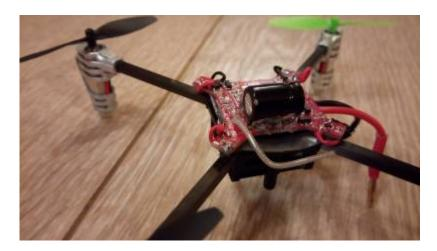
OK, the Cap is a little large, but was the only one with enough capacity I had laying around... Doesn't matter, It's not that heavy...
