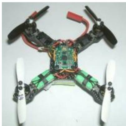
h8s-3d, using a 2mm round pin female micro connector
