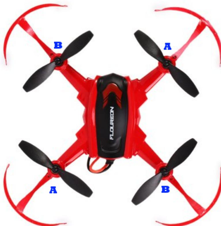
2. Motors/propellers are obstructed in some way. Check each propeller is spinning freely when flicked with your finger. Any that do not spin freely are at issue. Check that these are not pressed too firmly causing friction between the frame and the propeller. Also check for foreign objects such as hair or cobwebs, etc.
